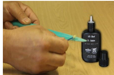
(Fig: 3) Cotton bud sparingly coats prop
